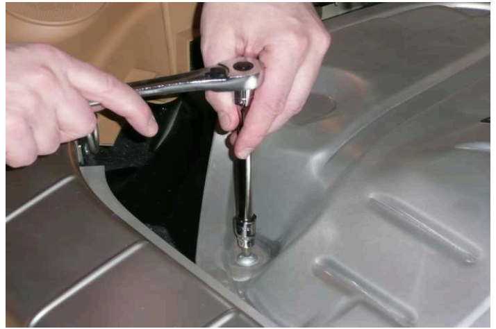
6. REMOVE ALL FIVE TORX-HEAD MACHINE SCREWS WITH A TORX T30 SOCKET DRIVE.
