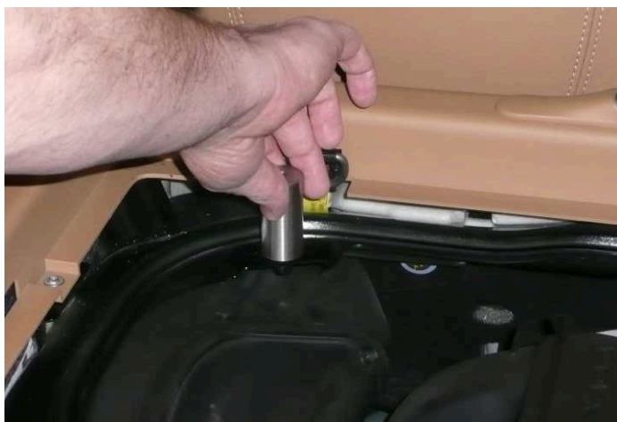
9. THREAD STEEL SPACERS INTO THE TWO FORWARD-OUTER METAL-COVER FASTENER LOCATIONS.
