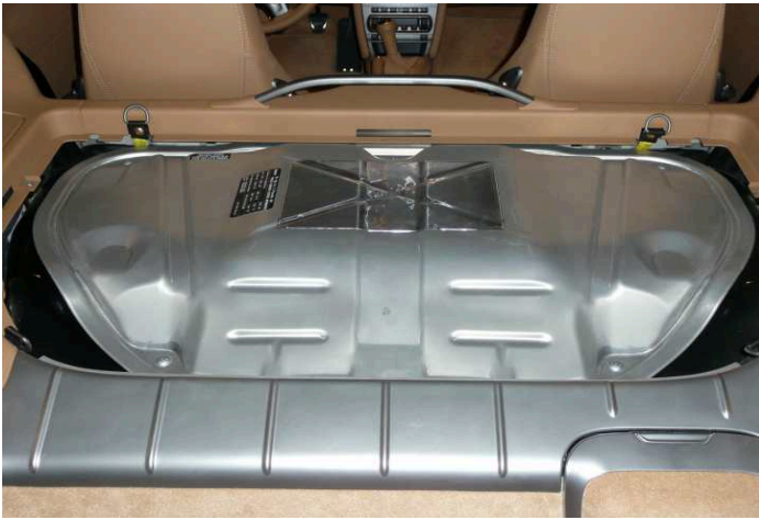
5. ALUMINUM ENGINE COVER, HELD IN PLACE WITH FIVE (5) TORX-HEAD MACHINE SCREWS.
