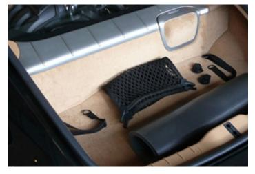
16. TO DISPLAY THE ENGINE, SIMPLY REMOVE THE FORWARD CARGO-NET ATTACHMENT FITTINGS BY PULLING UPWARD ON THE D-RINGS AND ROLL-UP (DO NOT FOLD OR CREASE) THE PROTECTIVE COVER WITH THE BLACK VINYL FACING OUTWARD. THE PROTECTIVE COVER CAN BE STOWED TEMPORARILY IN THE AFT TRUNK SPACE.
