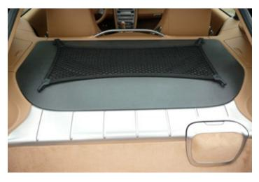
6. CARGO-NET SHOWN WITH THE TWO FORWARD HOOKS ATTACHED TO THE D-RING FITTINGS.
