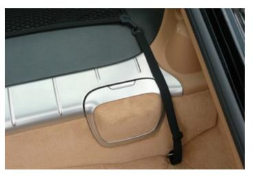
12. THE STRAPS ARE ADJUSTABLE. LENGTHEN THE STRAPS AND ATTACH THE CARGO-NET HOOKS TO THE STRAP D-RINGS.
