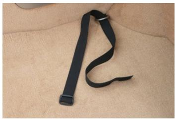
7. NOW BEGIN THE INSTALLATION OF THE AFT CARGONET ATTACHMENT-STRAPS BY INSERTING THE STRAPS THROUGH THE EXISTING D-RINGS IN THE LOWER TRUNK.
