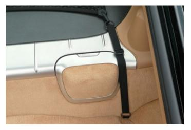
13. WITH THE CARGO-NET ATTACHED, ADJUST THE STRAPS TO TENSION THE CARGO-NET APPROPRIATELY.
