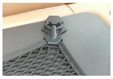
5. WITH THE CARGO-NET ATTACHMENT D-RING FITTINGS INSTALLED, ATTACH THE FORWARD HOOKS OF THE CARGO-NET TO THE D-RINGS.
