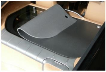
1. WITH THE HIP TRANSPARENT ENGINE COVER ALREADY INSTALLED, ROLL-OUT THE HIP PROTECTIVE COVER SO IT LAYS FLAT WITH THE SOFT CLOSED-CELL-FOAM (GREY SIDE) FACING DOWN AGAINST THE TRANSPARENT COVER. (BLACK VINYL FACING UP)
