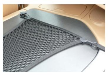
14. ICARGO-NET INSTALLED AND PROPERLY TENSIONED. ADJUST THE STRAPS TO ACCOMMODATE THE VARIOUS CARGO CAPACITY REQUIREMENTS.
