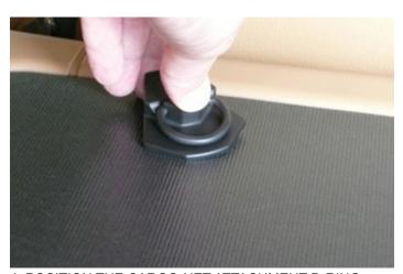
4. POSITION THE CARGO-NET ATTACHMENT D-RING FITTING SO THE D-RING WILL BE ALIGNED WITH THE CARGO-NET HOOK WHEN IT IS ATTACHED. PRESS THE FITTING DOWN SO THE BASE SITS FLAT ON TOP OF THE PROTECTIVE COVER.
