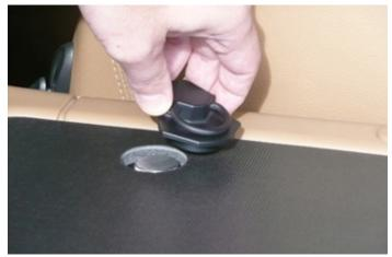
3. THE CARGO-NET ATTACHMENT D-RING FITTINGS ARE INSTALLED BY SIMPLY PRESSING THEM ON TO THE TOPS OF THE TRANSPARENT ENGINE COVER THUMB SCREWS.
